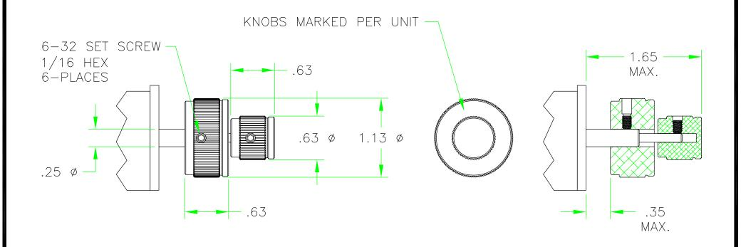
NOTE: PANEL THICKNESS IN ADDITION TO SCREW HEAD MUST NOT EXCEED .35 MAX.
