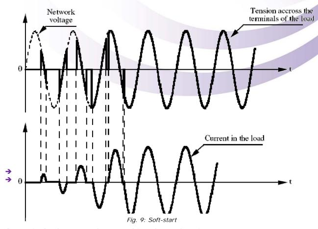
→ For single phase transformers, this softstart function can be built based on an analog proportional controller (e.g. SG4 series)
