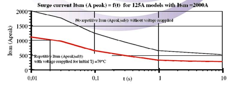
Fig. 6: 125 Solid-state relay ITSM curve
