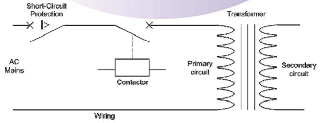
Frequent switching of the primary without adapted solution can lead to damages in the transformer primary circuit:
