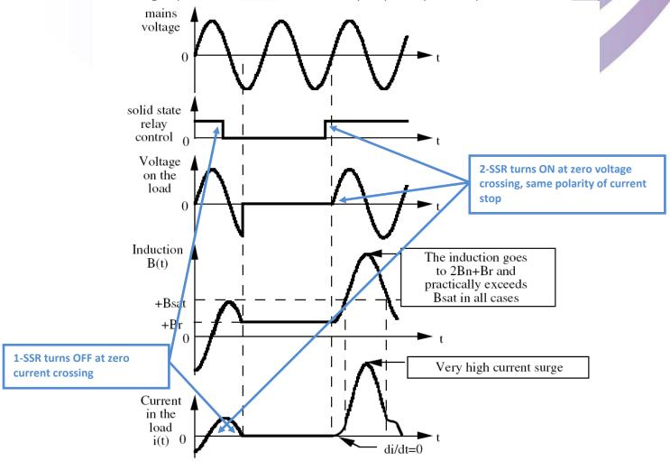
Fig. 4: zero cross switching, stop and start with same polarities
