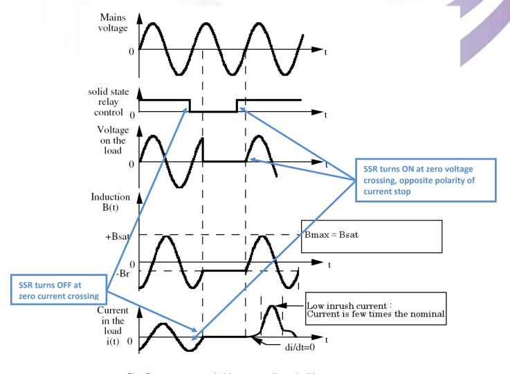
Fig. 5: zero cross switching, opposite polarities
