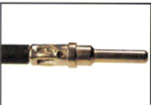
7. Inspect terminal to ensure that all strands are in crimp barrel. **NOTE:** Tool must be readjusted for each type/size of contact. Use HDT04-08 for size 8 and 4 contacts.
