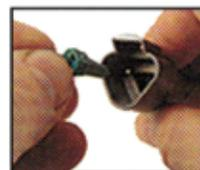
4. Once all contacts are in place, insert wedge lock. The wedge lock will snap into place. **NOTE:** The receptacle is shown. Use the same procedure for plug.
