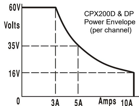
Operating Ranges: Four selectable ranges: 60V/10A, 60V/3A, 16V/10A and Custom Limits.
