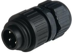
Circular Field Attachable Power Connector (CA Series): Male, straight, 4-pin(3+PE), integrated strain relief, 400 V AC/230 V DC, 16 A AC/10 A DC
