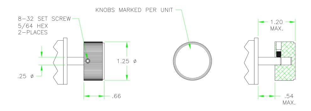
NOTE: PANEL THICKNESS IN ADDITION TO SCREW HEAD MUST NOT EXCEED .54 MAX.
