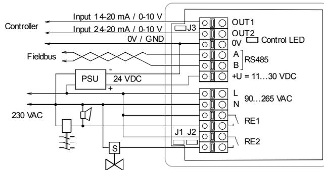
To power the instrument from an external 24 VDC source, connect terminals 0 V and +U to the source. If an integrated mains power supply module is used, connect terminals L and N to the mains.
