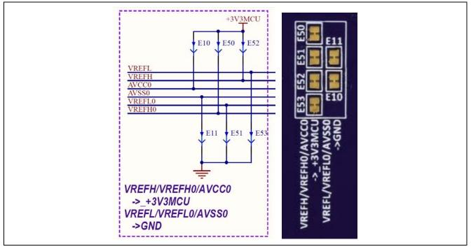
Figure 24. Analog and Reference Voltages
