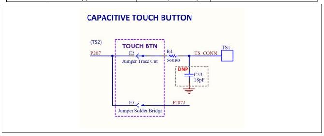
Figure 19. Capacitive Touch Button Circuit
