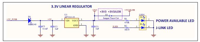
Figure 9. 3.3 V Power Regulator Circuit
