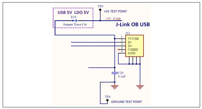
Figure 8. 5 V Power Input Circuit
