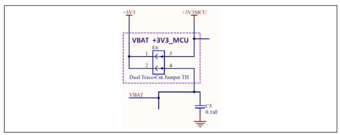
Figure 11. MCU Current Measurement Circuit
