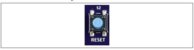
Figure 18. Reset Switch (S2) on the Target Board
