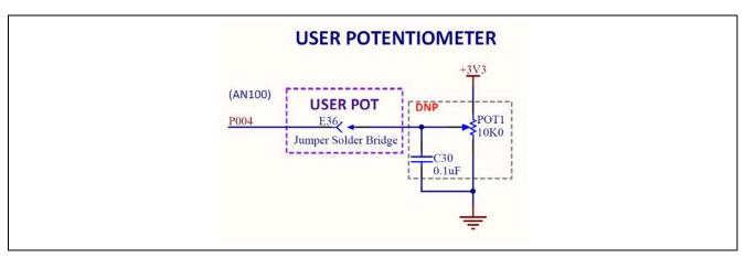
Figure 26. User Potentiometer Circuit
