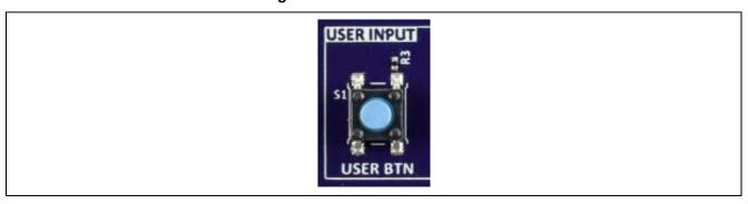
Figure 16. User Switch (S1) on the Target Board
