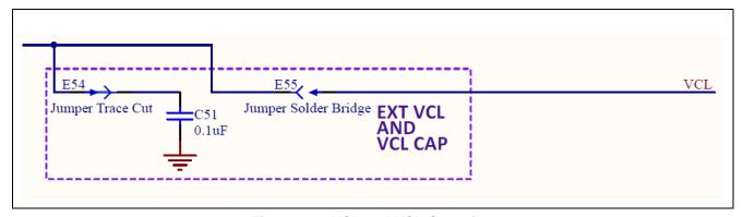
Figure 29. VCL and VCL Capacitor
