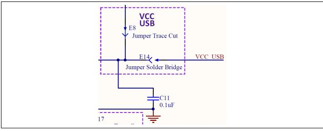
Figure 30. VCC\_USB Circuit
