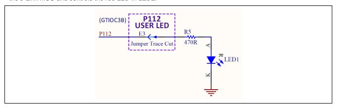
Figure 14. LED1 Control Circuit
