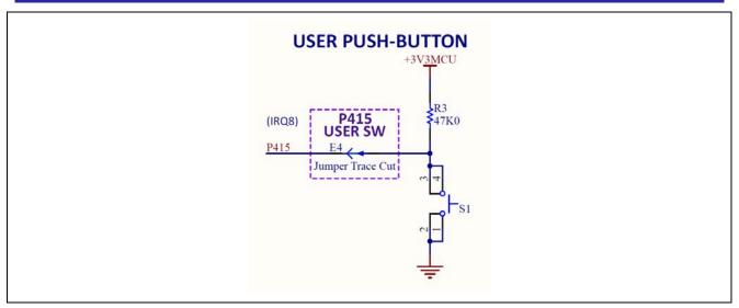
Figure 15. User Switch Circuit
