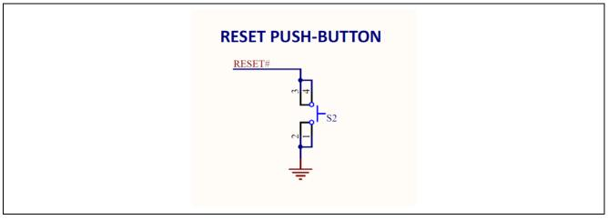
Figure 17. Reset Switch Circuit
