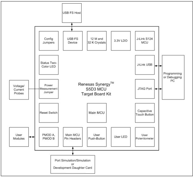
Figure 5. TB-S5D3 Block Diagram
