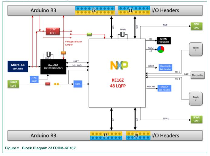
Figure 2. on page 3 shows the block diagram of the FRDM-KE16Z Freedom board.
