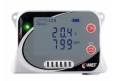
Datalogger is designed to record temperature, humidity and CO2. In case of exceeded set limits alarms are indicated by LED, LCD and acoustically by built-in beeper.
